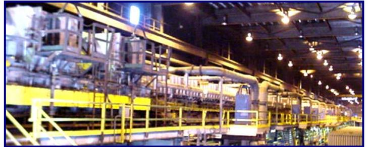
Because the furnace is cannot achieve abrupt changes in temperature, specific limits are placed on the scheduling of coils in order to ensure smooth transitions between products with different annealing requirements. Since the annealing process depends on both time and temperature, operators are able to ease the transitions by adjusting the speed of the line.
