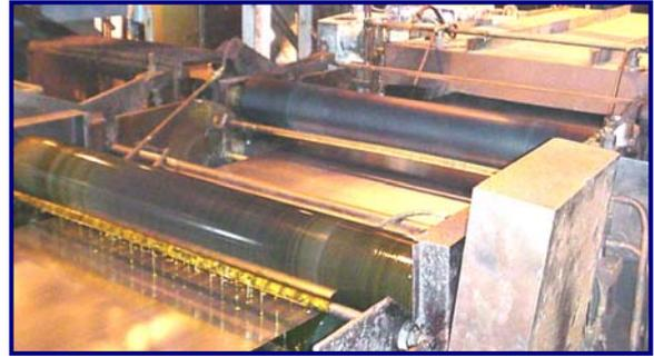
When indicated by the customer, the strip is oiled after inspection. A spreader roll at the #1 CGL squeegees oil evenly across the top surface of the steel shortly before it is recoiled, while the newer line uses an electrostatic oiler. Oil is less expensive than Chem Treat, but it is not as durable and is more difficult for the customer to clean from the strip. Typically, galvanize products that will be painted are oiled, while end-uses calling for exposed zinc receive Chem Treat.
